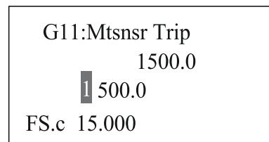
Third line: the user input empty pipes alarm threshold.
