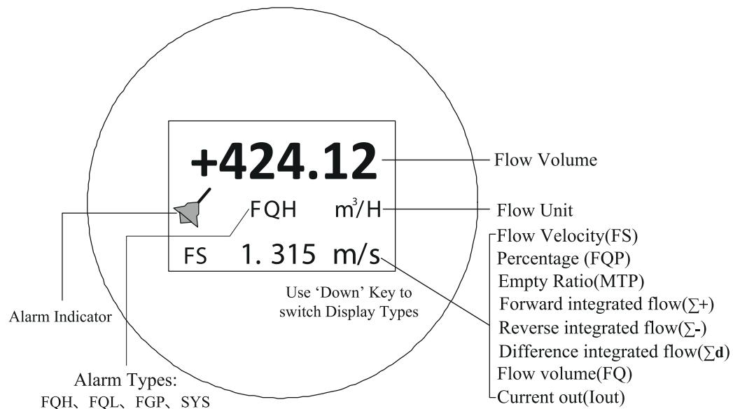
Note: When there more than one alarm, the alarm status display cycle.
